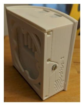
When you unpack your Terminal you will notice that the Case and the Wall Mount are screwed together. To install your Terminal you will have to remove the M3x5 screw and slide the Wall Mount out.
